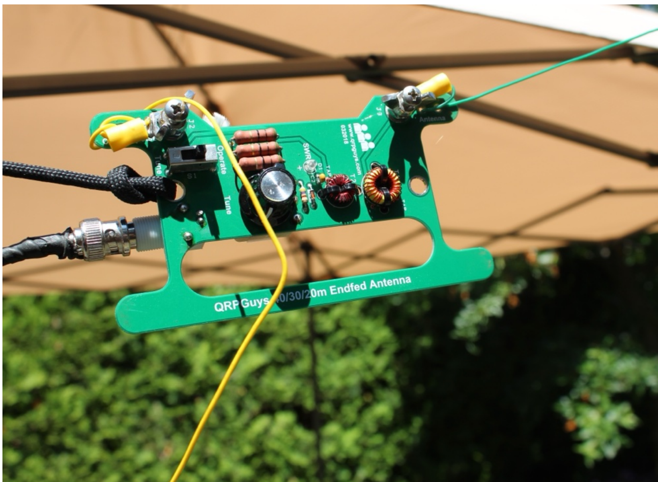
Figure 11. The QRguys end-fed antenna kit with matching network with RG-8 and antenna wire.
